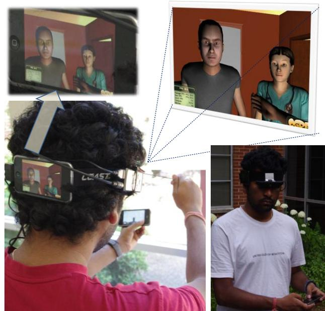
Figure 1 A user operating a UCAVE implementation inside and outside featuring a lightweight head-mounted display, smart phones and immersive 3D rendering.
